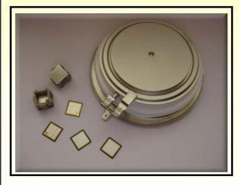
IXYS UK Westcode Ltd. announces the launch of its first 1.7kV press-pack IGBT. The new device is reverse conducting, with a fully rated diode integrated in the package and represents the first in a planned range of 1.7kV devices. The new device has a DC current rating of 960A and repetitive peak collector current of 1920A, with a continuous DC rating of 900V.
